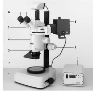
Fig. 4 Right side of the Leica MZ16 F
